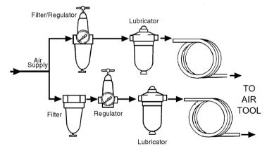
A typical air line layout is shown above. If an automatic in-line filter/regulator is used, it will keep the tool in good condition, but should be regularly checked.
